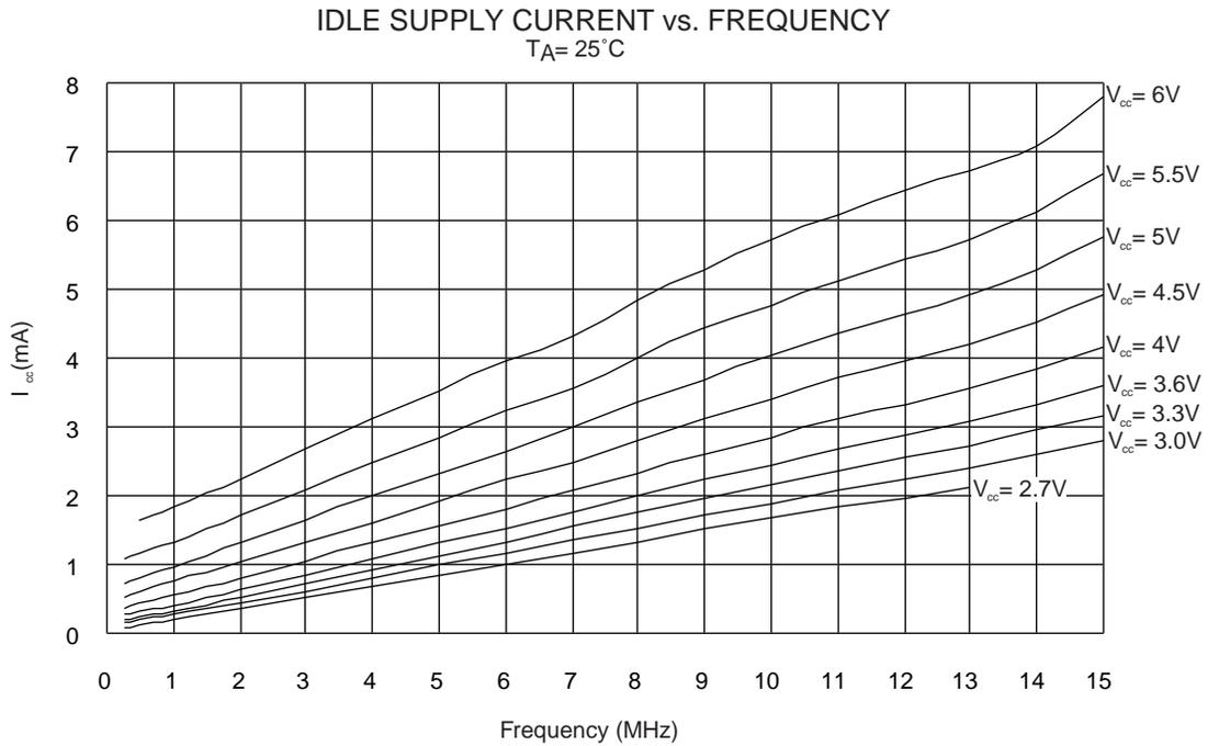
Figure 60. Idle Supply Current vs. V<sub>CC</sub>
