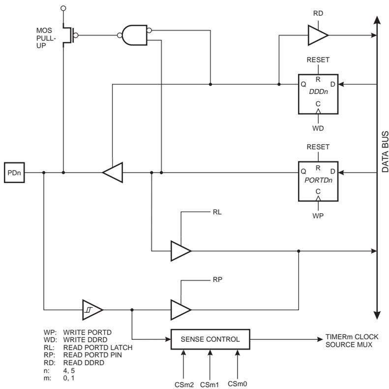
**Figure 48.** Port D Schematic Diagram (Pin PD6)
