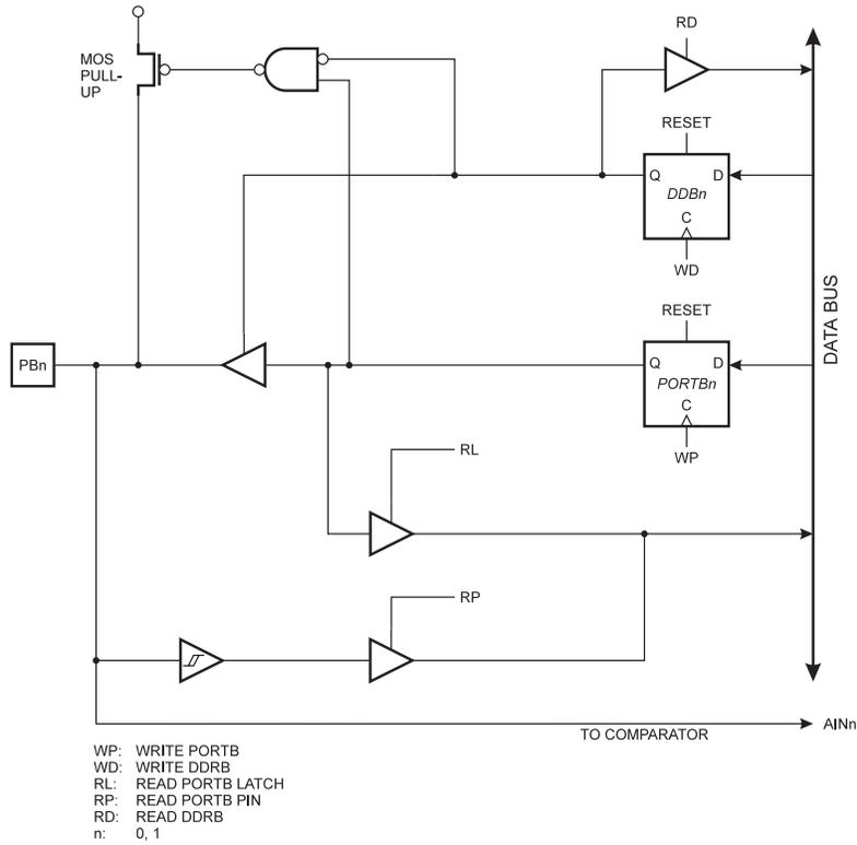
**Figure 39.** Port B Schematic Diagram Pin PB3
