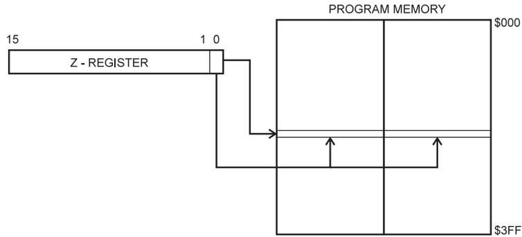
Constant byte address is specified by the Z-register contents. The 15 MSBs select word address (0 - 1K), the LSB selects low byte if cleared (LSB = 0) or high byte if set (LSB = 1).
