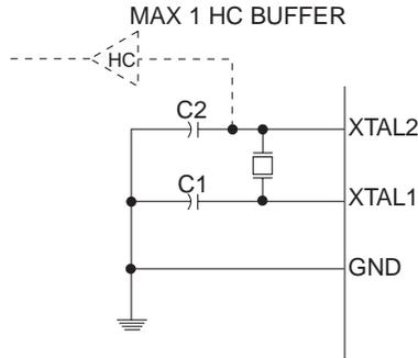
Note: When using the MCU Oscillator as a clock for an external device, an HC buffer should be connected as indicated in the figure.
