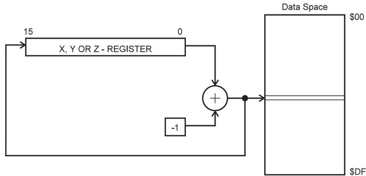
The X, Y or the Z-register is decremented before the operation. Operand address is the decremented contents of the X, Y or the Z-register.
