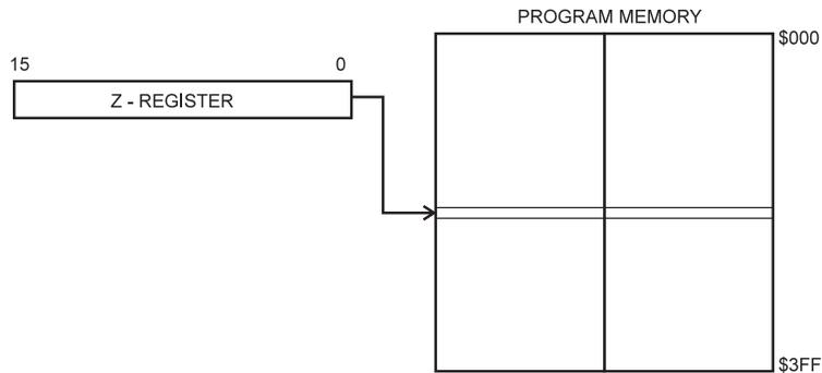
Program execution continues at address contained by the Z-register (i.e., the PC is loaded with the content of the Z-register).
