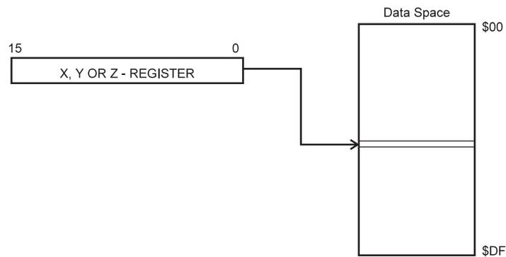
Operand address is the contents of the X, Y or the Z-register.
