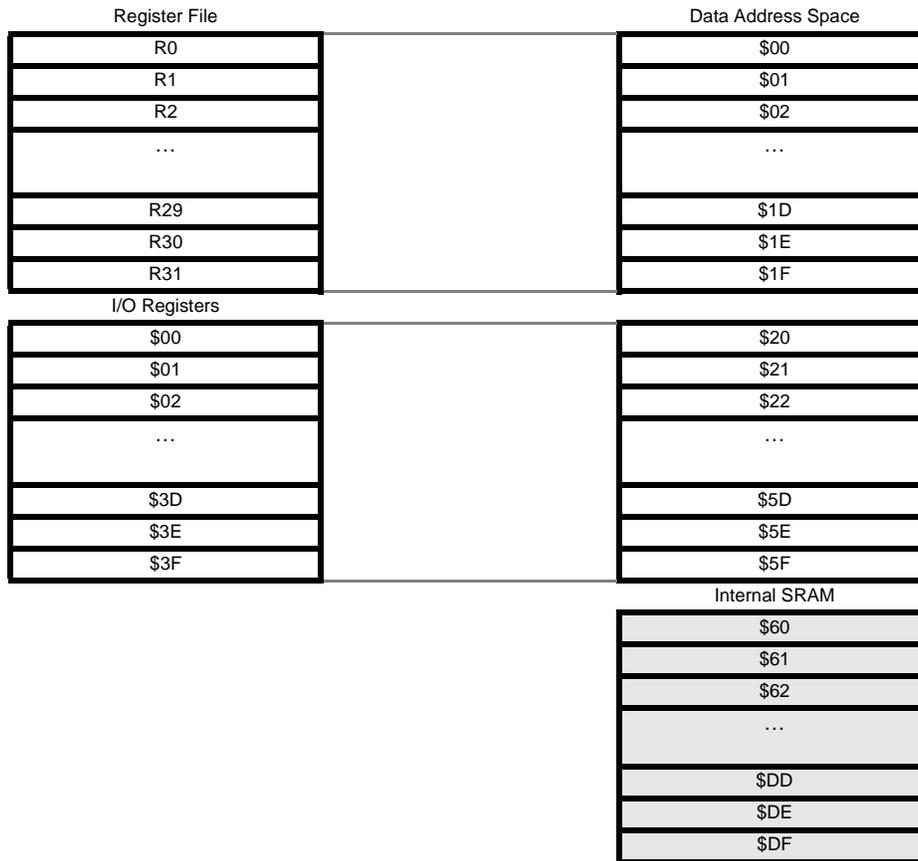
The 224 Data Memory locations address the Register file, I/O Memory and the data SRAM. The first 96 locations address the Register File + I/O Memory, and the next 128 locations address the data SRAM.
