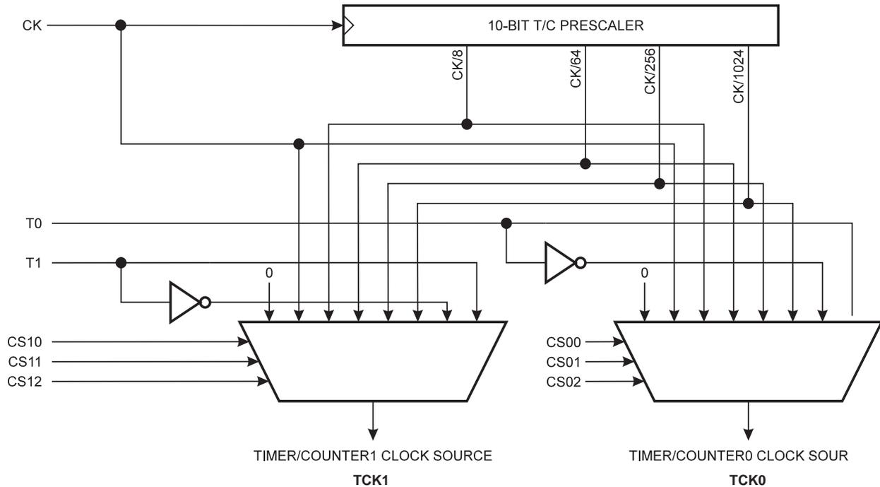
The four different prescaled selections are: CK/8, CK/64, CK/256 and CK/1024 where CK is the oscillator clock. For the two Timer/Counters, added selections as CK, external clock source and stop, can be selected as clock sources.
