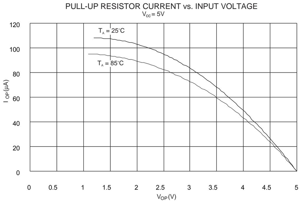
**Figure 69.** Pull-Up Resistor Current vs. Input Voltage
