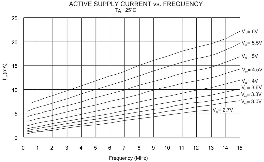
**Figure 58.** Active Supply Current vs. V<sub>CC</sub>
