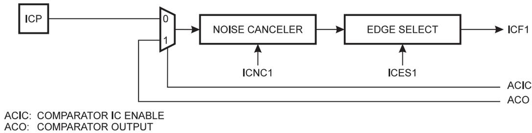
If the noise canceler function is enabled, the actual trigger condition for the capture event is monitored over 4 samples, and all 4 must be equal to activate the capture flag.
