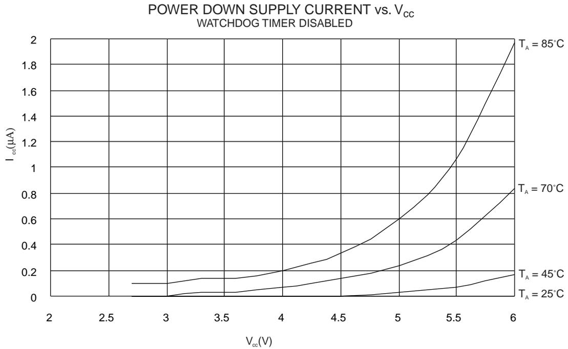
**Figure 62.** Power Down Supply Current vs.  $V_{CC}$
